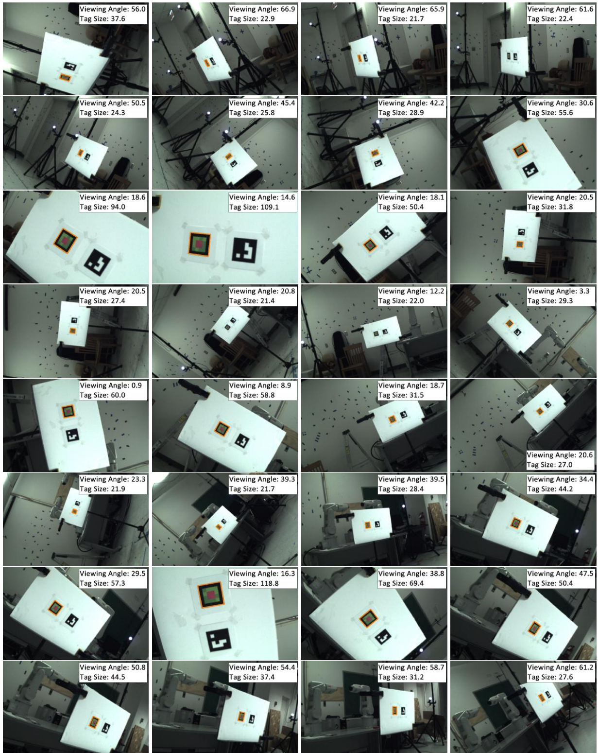
Figure 3.9: Example images processed by ChromaTag with labeled tag size and viewing angle.
