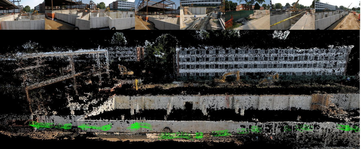
Figure 5.6: The scene scale dataset consists of 160 images of a construction site with an accompanying point cloud, normal vectors, and camera intrinsic and extrinsic parameters. The SFM-registered camera frusta are shown in green. 11 of the 19 material categories are represented: “Brick”, “Cement – Smooth”, “Concrete – Precast”, “Concrete – Cast in Place”, “Foliage”, “Grass”, “Gravel”, “Metal – Grills”, “Soil – Compact”, “Soil – Loose”, and “Wood”.
