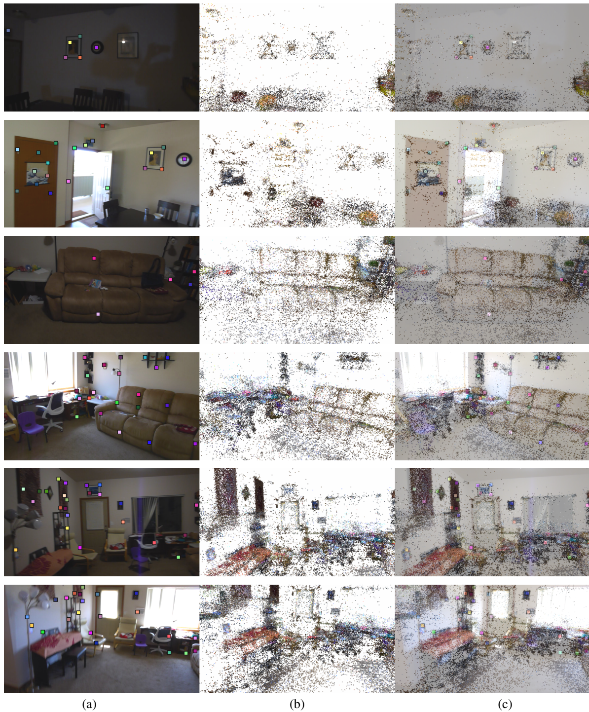
Figure 10. Qualitative results (scene5) : Each row shows (a) a query image from the test set with SLD landmark detections (shown as colored squares); (b) the rendering of the SfM point cloud obtained from training images, projected using the camera pose estimated by our proposed NBE+SLD method; and (c) an overlay of the rendering on the query image. The point cloud is not used by our method. They are rendered only for the purpose of visualization to assess the accuracy of the pose estimate. These images show SLD detections on the same objects and surfaces (photographs, wall hangings, sofa, door corner) in different images where the lighting varies considerably.
