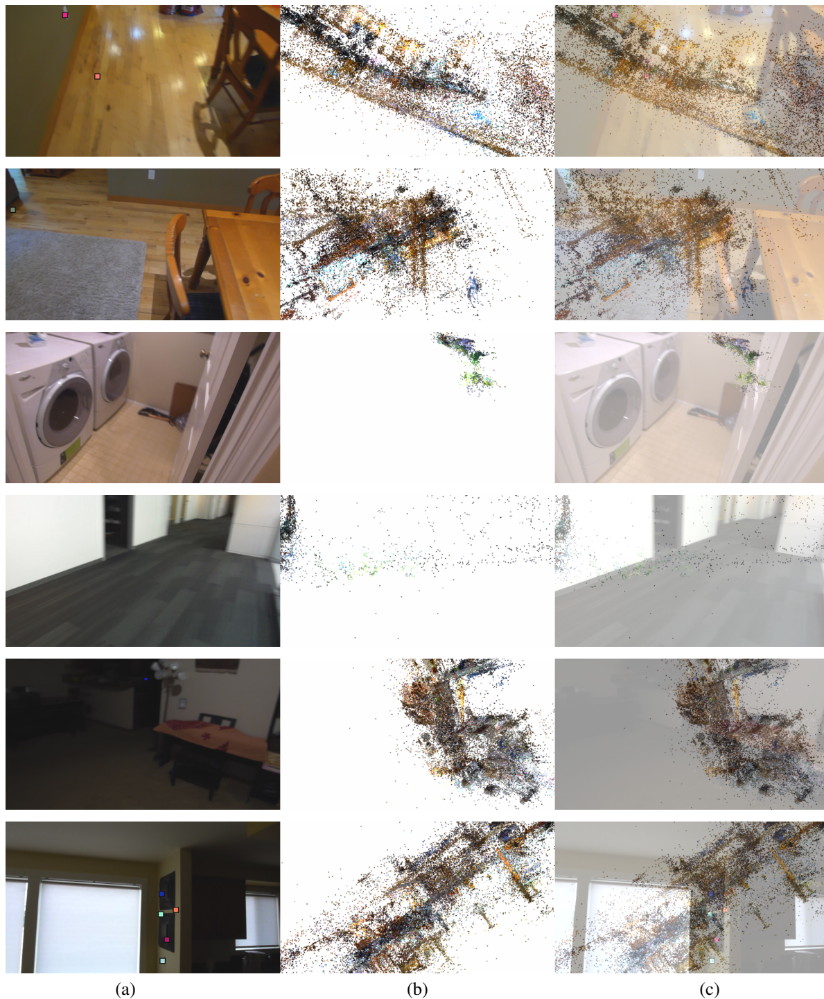
Figure 12. Failure Examples: Each row shows (a) a query image from the test set with SLD landmark detections (shown as colored squares); (b) the rendering of the SfM point cloud obtained from training images, projected using the camera pose estimated by our proposed NBE+SLD method; and (c) an overlay of the rendering on the query image. The point cloud is not used by our method. Our method can be inaccurate when a sufficient number of landmarks are not detected and NBE bearing predictions are also not accurate enough. Some failures are shown (top to bottom) – insufficient landmarks and too few training images observing floor (scene2), laundry room (scene1), and hallway (scene6); too dark (scene5); and high dynamic range-induced false detections (scene3).
