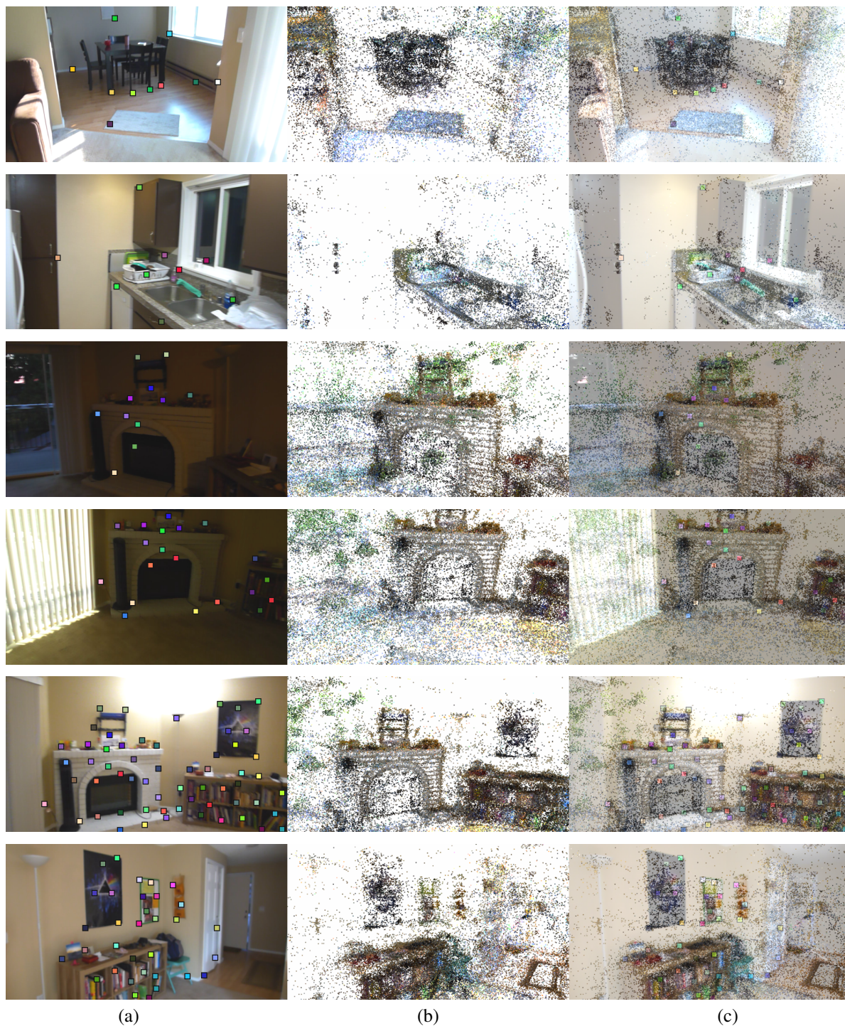
Figure 6. Qualitative results (scene1) . Each row shows (a) a query image from the test set with SLD landmark detections (shown as colored squares); (b) the rendering of the SfM point cloud obtained from training images, projected using the camera pose estimated by our proposed NBE+SLD method; and (c) an overlay of the rendering on the query image. The point cloud is not used by our method. They are rendered only for the purpose of visualization to assess the accuracy of the pose estimate. The images contain dramatic illumination changes in this scene, ranging from strong sunlight to low-light at night. Our method detects several landmarks despite the lighting variations.
